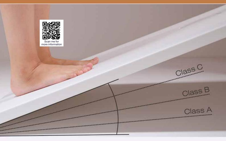
Exceeds Class C for DIN 51097 - Barefoot ramp test.
